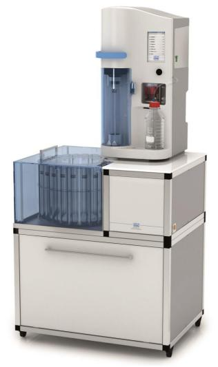
The UDK 169 Distillation & Titration System is designed to perform nitrogen and protein determination according to the Kieldahl Method (TKN) in the Food & Feed industries and several other applications in environmental control (phenols, nitrogen in water, sludge, soil and lubricant) and also in the chemical and pharmaceutical industries after having digested the sample accurately.
